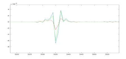
Figure 4: One trace comparison magnifying the event in figure 3 between 3.2s-3.5s. Red line: Data with Q. Green line: Data with Q after Q compensation. Blue line: Data without Q
