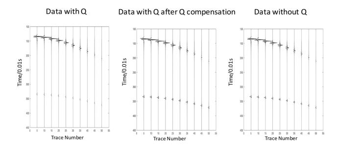
Figure 2: Left: Data generated by the model with Q. Middle: The data (with Q) after ISS Q compensation without knowing or estimating Q Right: Data generated by the same model but without Q.
